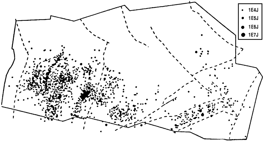
FIG. 21. Distribution of seismic events with magnitude greater than 1.2 recorded between 1990 and 1995 at Kleofas coal mine, Poland. Dashed lines mark tectonic faults. [Mutke and Stec (1997), Fig. 3, reprinted from Rockbursts and Seismicity in Mines , Proceedings of the 4th International Symposium, Krakow, Poland, 11–14 August 1997. 450 pp., EUR 137.50/US $162.00/GBP97.00, A. A. Balkema, P.O. Box 1675, Rotterdam, Netherlands.]
